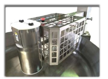
[Safety Measure] The stirring section is equipped with a safety cover and a torque limiter to prevent it from aettina cauaht.
